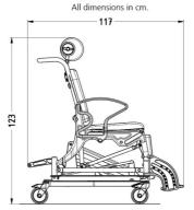
Rebotec Phoenix Multi in standard configuration includes seat with hygiene opening, adjustable headrest, bucket and bucket device and a charging charging station with second, backup battery. The chair is certified class IP56 (protected from limited dust ingress, protected from high pressure water jets from any direction).
